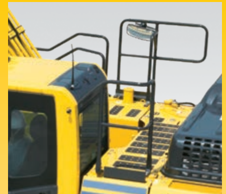
Hand rails and anti-slip plates
