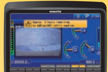
AdBlue® level and refill guidance
