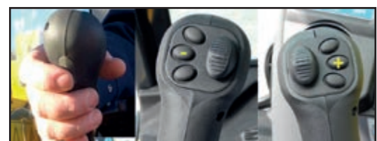
Right hand lever trigger switch for semi-auto function. Design offset +/- using lever button
