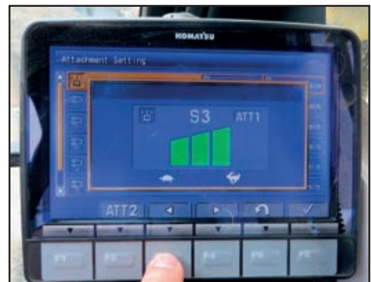
Adjustable pre-set flow options for smooth precise tilt operation. HCU A hydraulic circuit is used for tilt function.
