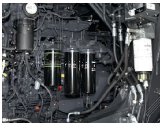
Centralized greasing points and filter arrangements make maintenance easier
