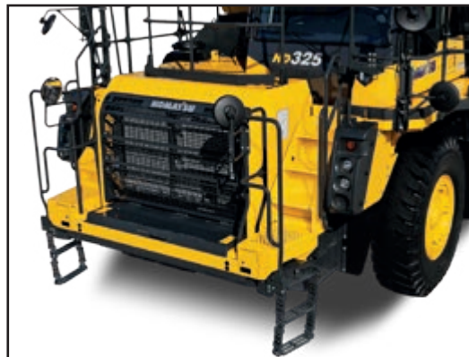
Safe and convenient cab access thanks to stairway with handrail
