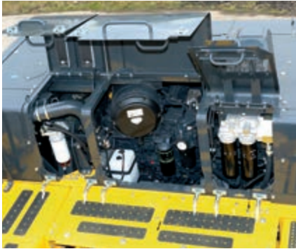
Easy access to filters on the front side of the engine hood
