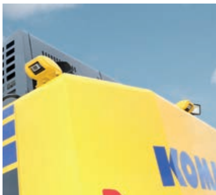
Rear-view and optional side-view camera
