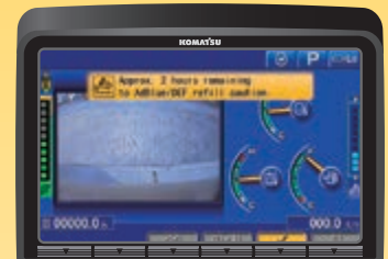
AdBlue® level and refill guidance
