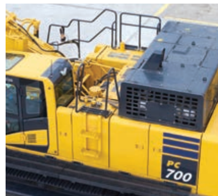
Hand rails and anti-slip plates
