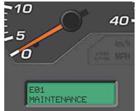
EMMS (Equipment Management Monitoring System)
