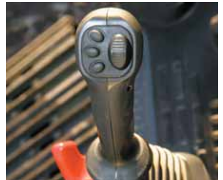
Joysticks with proportional control button for attachments
