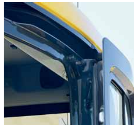
The sliding door facilitates easy entrance in confined areas while reducing the risk of damage on roadways. The cab also features a sliding window.
