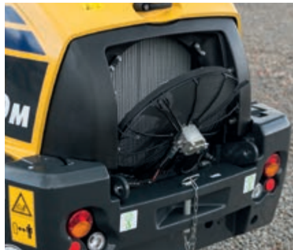
Tiltable radiator fan for convenient cleaning access
