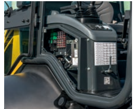
Side cover for quick maintenance access
