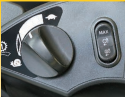
Variable shift control dial with creeping speed range (left) and variable traction control system switch (right)
