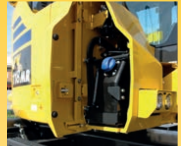
Simple access to the AdBlue® tank
