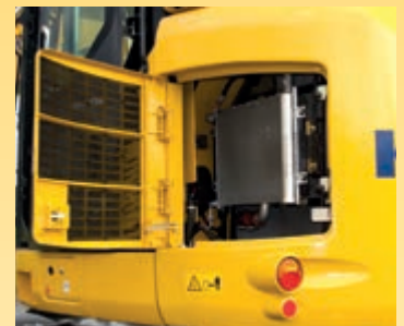
The cooler nets are integrated in the side doors for easy cleaning access from ground level
