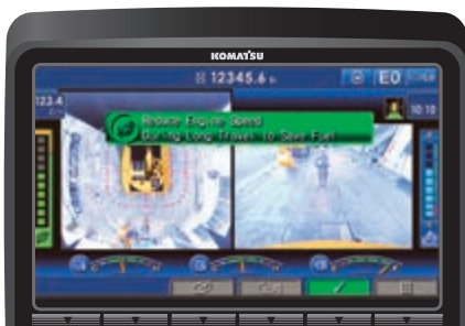
Eco-gauge, Eco guidance and fuel consumption gauge
