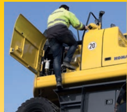
Handrails and anti-slip plates
