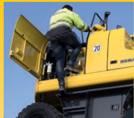
Handrails and anti-slip plates
