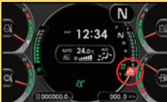
AdBlue® level gauge and refill guidance
