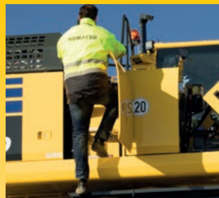
Straight ladder for service access, handrails and anti-slip plates
