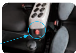
Secondary engine shutdown switch
