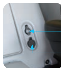
Cigarette lighter (DC 12 V) AUX terminal DC 12 V electrical outlet
