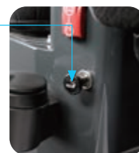
Cigarette lighter (DC 12 V) AUX terminal DC 12 V electrical outlet
