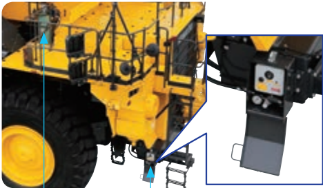
Grease pump and reservoir Refill port
