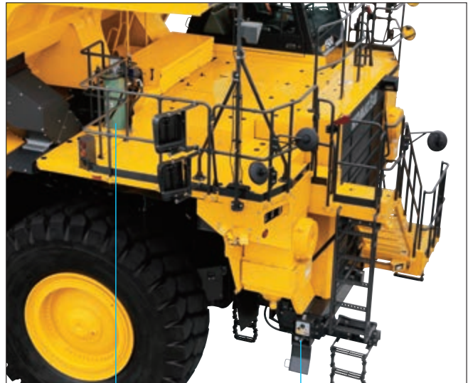
Grease pump pump and reservoir Refill port
