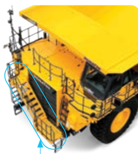
Dimpled slip-resistant plates are used
