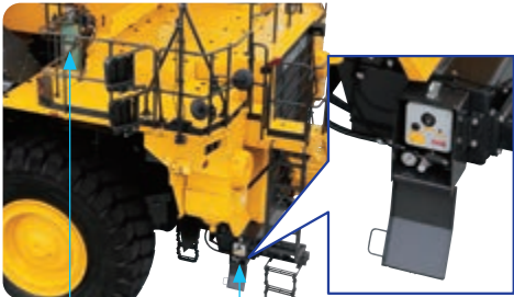
Grease pump and reservoir Refill port
