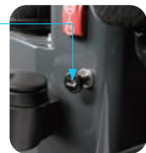
Cigarette lighter (DC 12 V) AUX terminal DC 12 V electrical outlet
