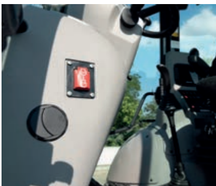
Secondary engine shut down switch
