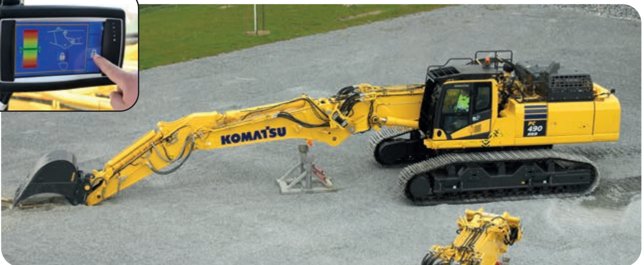
K100 quick boom change system (option) Includes Komatsu hands free boom connections, with advanced human machine interface safety system. Low profile equipment storage stands included.
