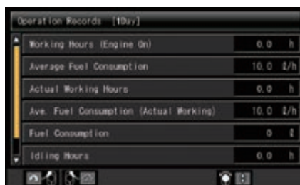
A multifunction monitor displays and controls a wealth of operational and maintenance information
