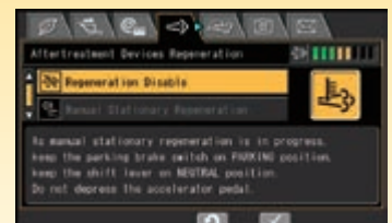
Aftertreatment device regeneration screen for the KDPF
