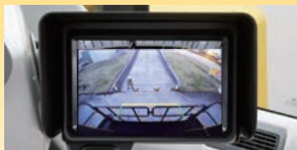
The Komvision system is separated from the rear-view monitor, which even uses a different camera.
