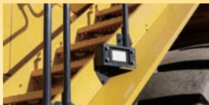
KomVision radar (optional) detects obstacles around the machine, displays them on the monitor screen and sounds a warning buzzer.
