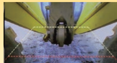
The front camera is located between the wheels and allows the operator to avoid driving over obstacles such as rocks, which may damage the tyres.
