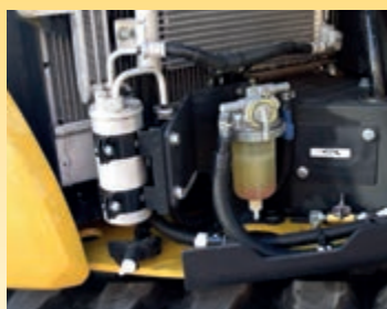
Large fuel filter and fuel pre-filter with water separator protect the engine
