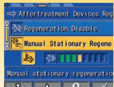
Aftertreatment device regeneration screen for the DPF
