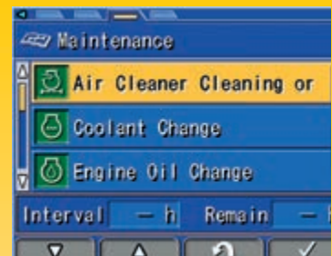
The updated multifunction monitor panel provides the operator with maintenance and service information
