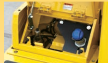
For simple access, the AdBlue® tank is installed on the front stairway.
