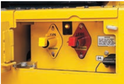
Battery and starter isolator box with jump start receptacle.
