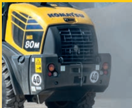
Wide core radiator with (optional) reversible fan
