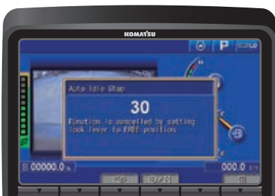
Eco gauge, Eco guidance, an adjustable idle shutdown and a new auto idle function all contribute to further reduce fuel consumption
