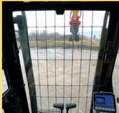
Carefully aligned grid layout ensures maximum visibility with correct protection. One piece front screen fitted with high impact protective glass.
