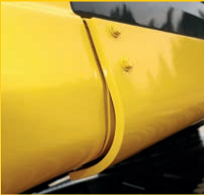
Extra heavy duty, wrap around type side protection (15 mm). Bolted to each side of the upper structure, offering protection from debris on the ground or side impact.
