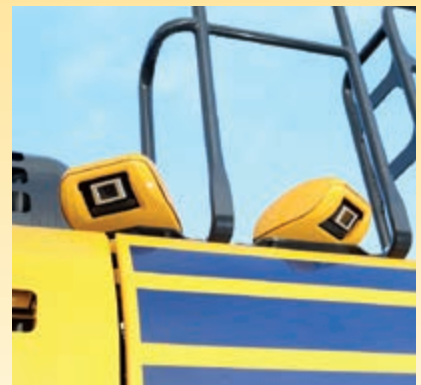
KomVision machine visibility gives the operator a constant clear view of the safety zone around the machine. This allows the operator to focus on the work at hand even in low light conditions.
