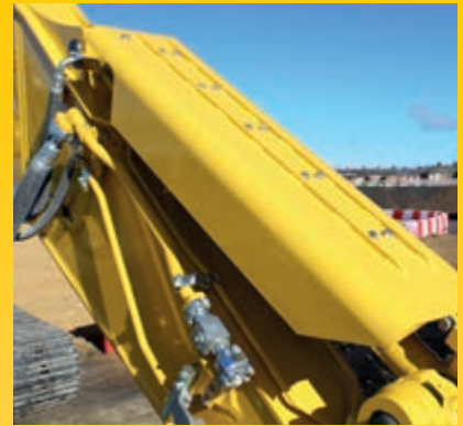
Attachment cylinder guard (option), reinforced bucket linkage and details like heavy duty boom lamp protection guards round up the all-round protection.
