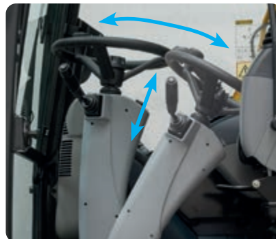
The standard telescopic steering wheel is comfortably adjustable in height and reach
