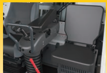
The standard trainer seat can be folded up when not in use.
