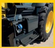
AdBlue®, fuel and hydraulic oil tank are easily accessible on the machine side and refilled by ground level, ensuring a fatigue less operation
