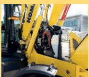
Daily maintenance is enhanced thanks to the double position front opening and the check point position easily accessible on the left side
