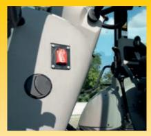
Secondary engine shut down switch
